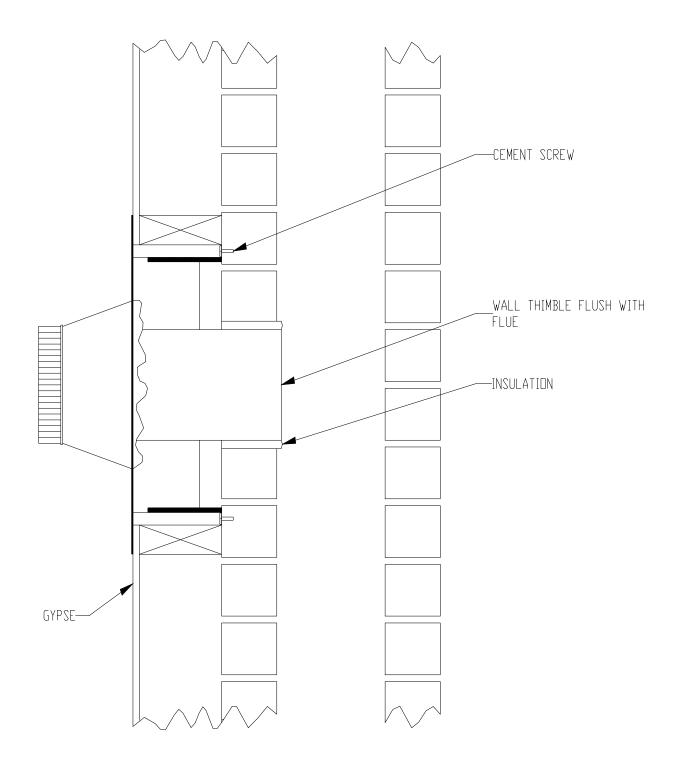
FIGURE 2.2.2 (B) Factory Built Thimble
